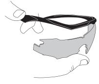
5) Detach the outer lens hooks from the frame.
