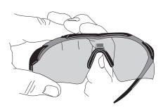
2) Position hand as pictured and squeeze together until the nose piece completely seats into the lens.
