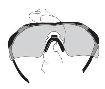
1) Align grooves of nose piece into the lens.
